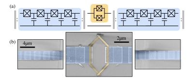
This is an example of a high-impedance superconducting circuit that we use to observe dual Shapiro steps. We use chains of thousands of Josephson junctions (in blue) to create high-impedance environments for ultra-small Josephson junctions (in yellow). As a result, these smaller junctions operate in the charge regime rather than the usual phase regime. This allows them to host Bloch oscillations, which are the dual of the well-established Josephson oscillations.
